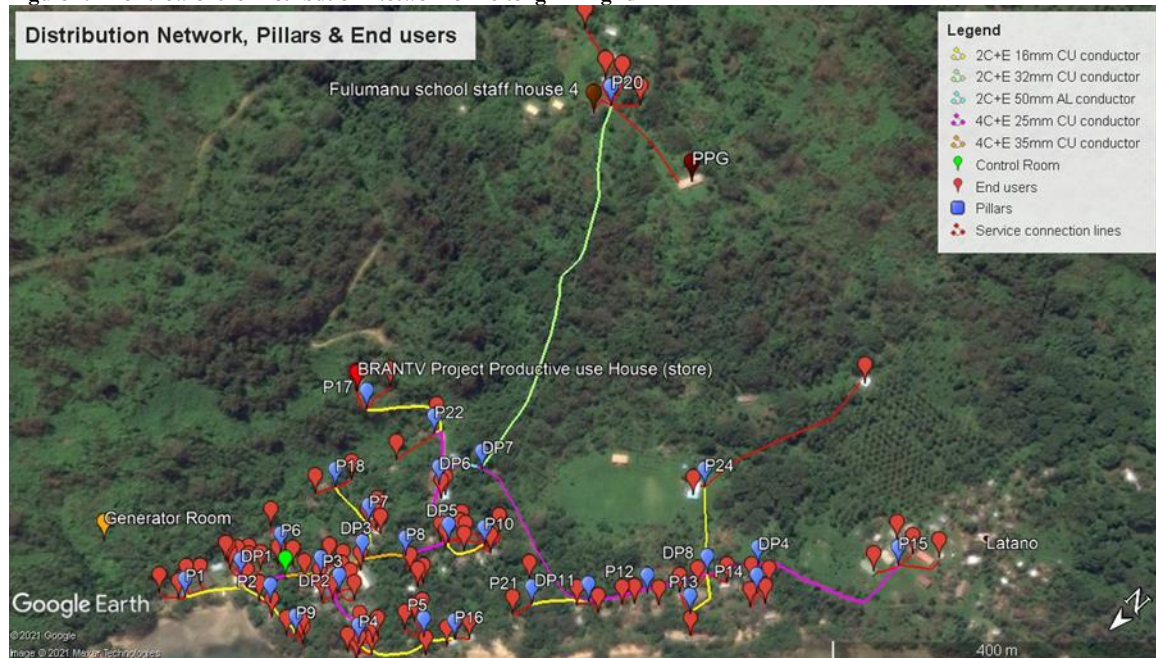
Figure 2: Ariel View of the Distribution Network of Lolong Mini grid
